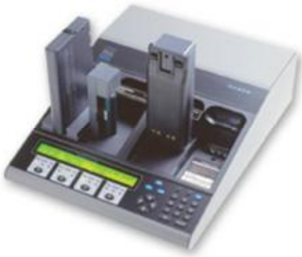
Our in-house CADEX C7400 Battery Analyser Station
